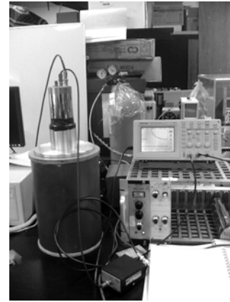
Fig.2: Scintillator and PMT in a plastic cylinder
